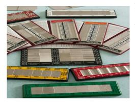
Electroforming in nickel has been found to be the only method by which secondary standards can be made with the same degree of surface precision as the primary standard, at a lesser price. These standards are essential to achieve the high standards of surface precision required by modern engineering industry
