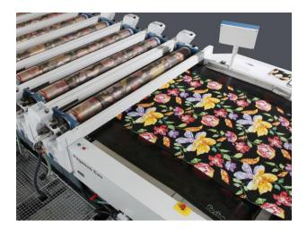
The technology involves transferring the inks of different colours that make up the decorative patterns to the substrate materials through perforated metallic rotating cylinders as shown alongside
