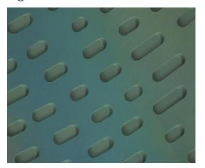
At this stage of the development of the discs the depressions would typically be 0.2 µm deep by 0.4  $\mu$ m wide by 1.6  $\mu$ m long. The information is carried bv variation in the depression length. A disc would typically have 30,000,000,000 depressions on its surface all of which must be the correct length, depth and width and in exactly the right position on the disc surface.
