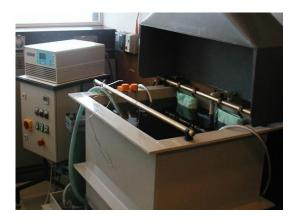
The most significant development in electrolytic nickel deposition processes appeared in 1916 when Oliver Watts published his work defining the composition of a solution based on nickel sulphate with additions of nickel chloride and boric acid. The 'Watts Solution', as it became universally known, has remained the mainstay of the nickel electroplating industry for the last 95 years.
