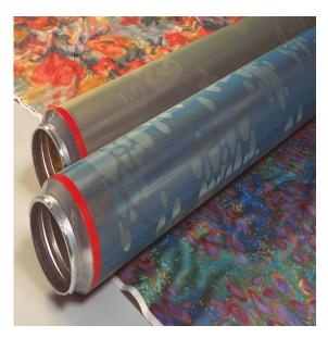
In order to produce the required printing patterns, cylinders are manufactured with billions of tiny holes in their walls, ranging in size from 0.6 mm. down to 0.08 mm. in diameter.
